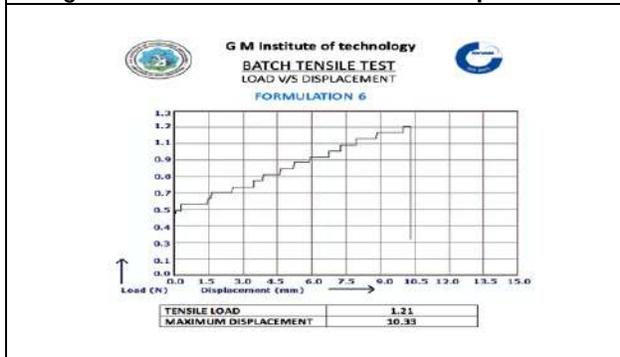
Figure 9. Tensile Load vs Maximum Displacement
