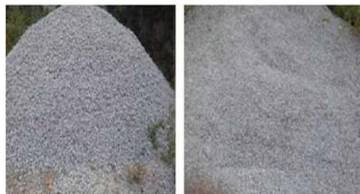
**Fig 2 :20mm and 12mm Coarse Aggregates**
