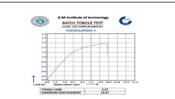
Figure 4. Tensile Load vs Maximum Displacement
